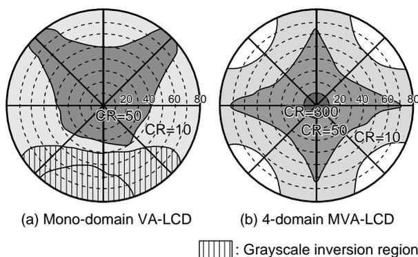
Figure 5 Viewing angles of VA and MVA-LCD.
