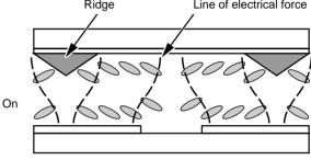
Figure 8 Structure combining a slit and ridges.
