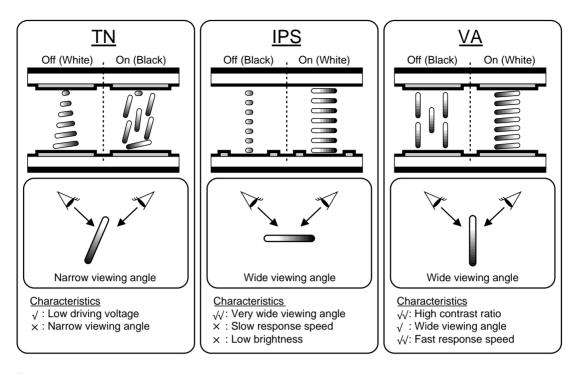
Figure 1 Comparison of liquid crystal display modes.
