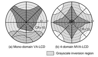
Figure 5 Viewing angles of VA and MVA-LCD.
