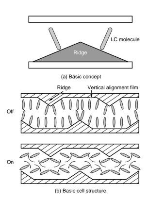
Figure 3 Operating principle of MVA-LCD.
